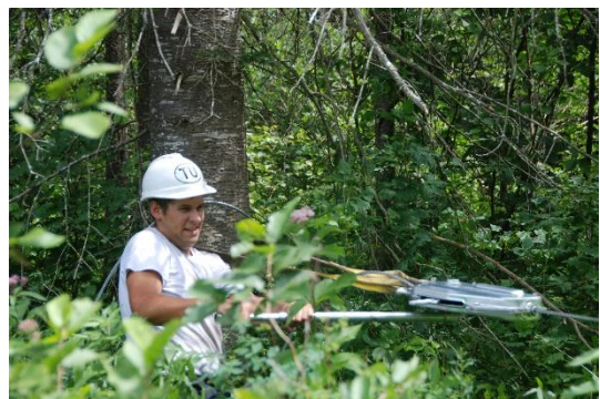
Figure 1. The chop-and-grip technique utilizes a grip hoist to secure downed trees.
